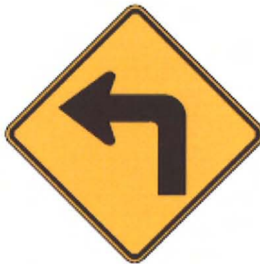
HORIZONTAL ALIGNMENT WARNING SIGN W1-1
