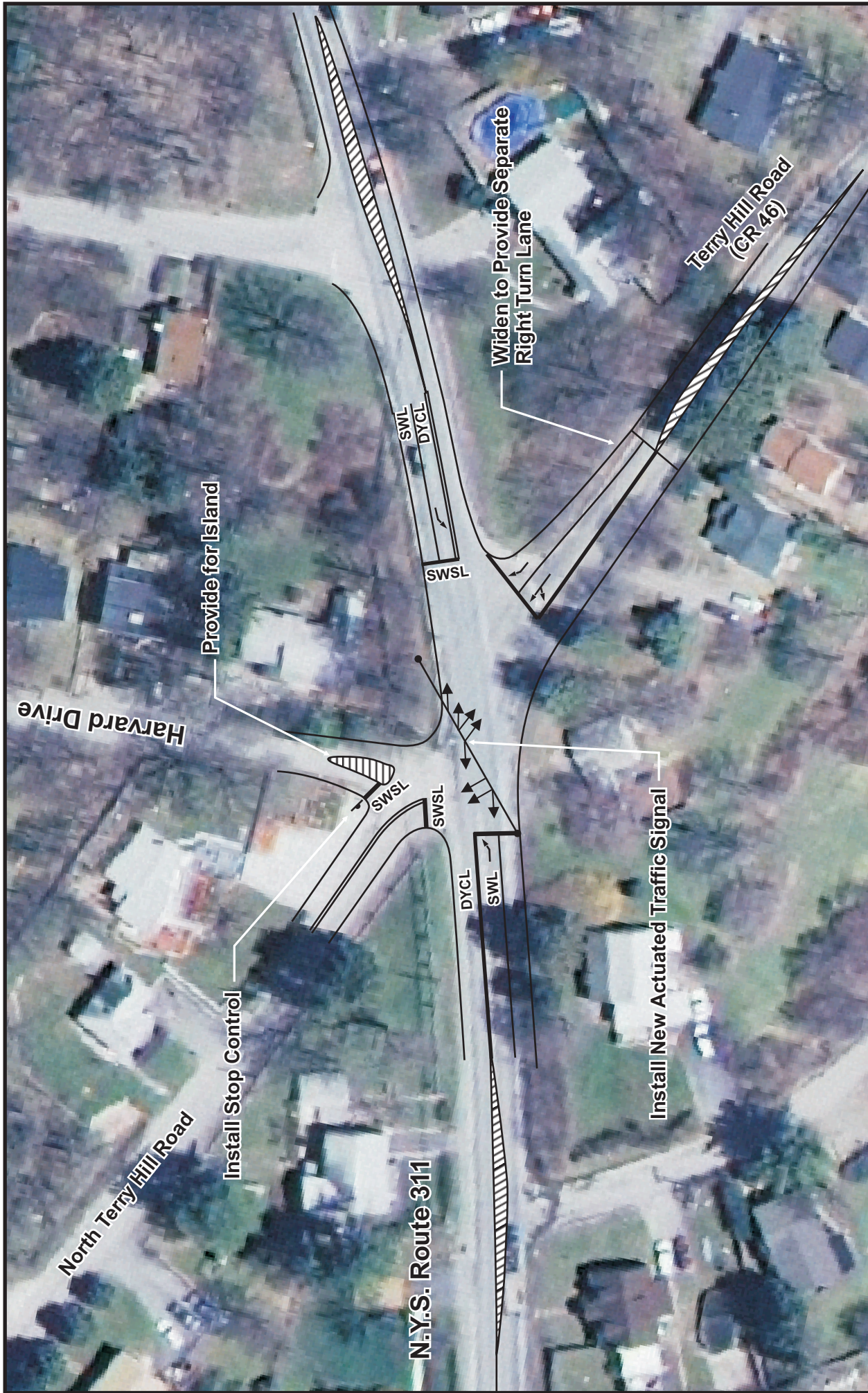
Figure K-2: Potential Improvement Schematic Terry Hill Road/NYS Route 311 Concept Plan for Potential Improvements Patterson Crossing Retail Center Town of Patterson and Town of Kent, Putnam County, New York Source: John Collins Engineers, P.C., 6/18/07 Scale: 1" = 65'
