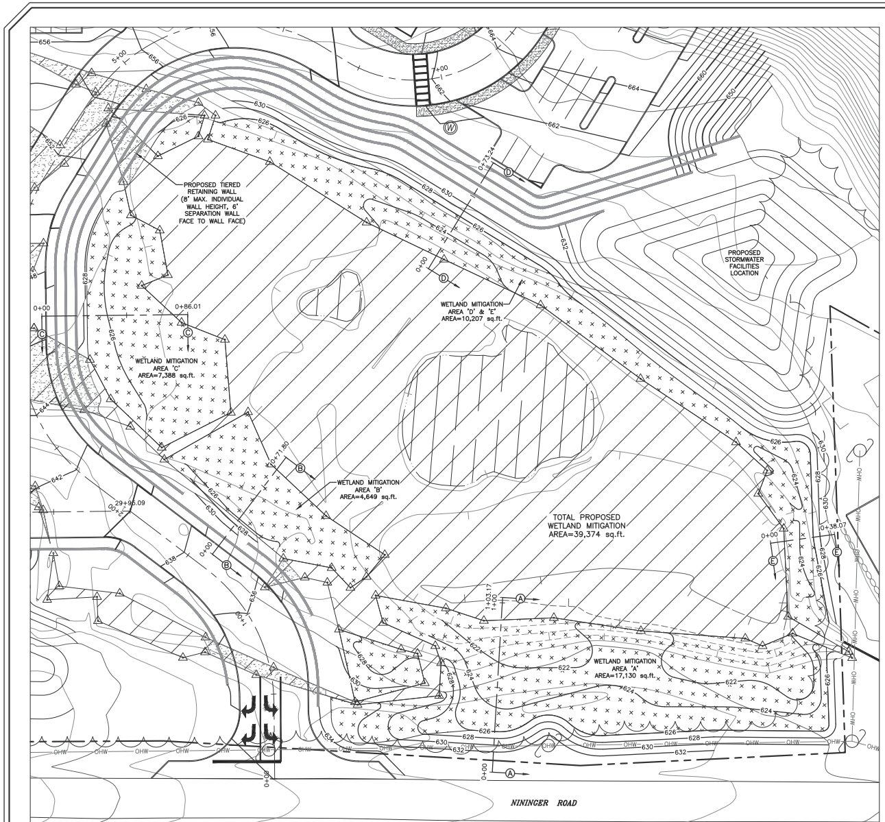
FEDERAL WETLAND MITIGATION AREA - GRADING PLAN SCALE: 1" = 50'
