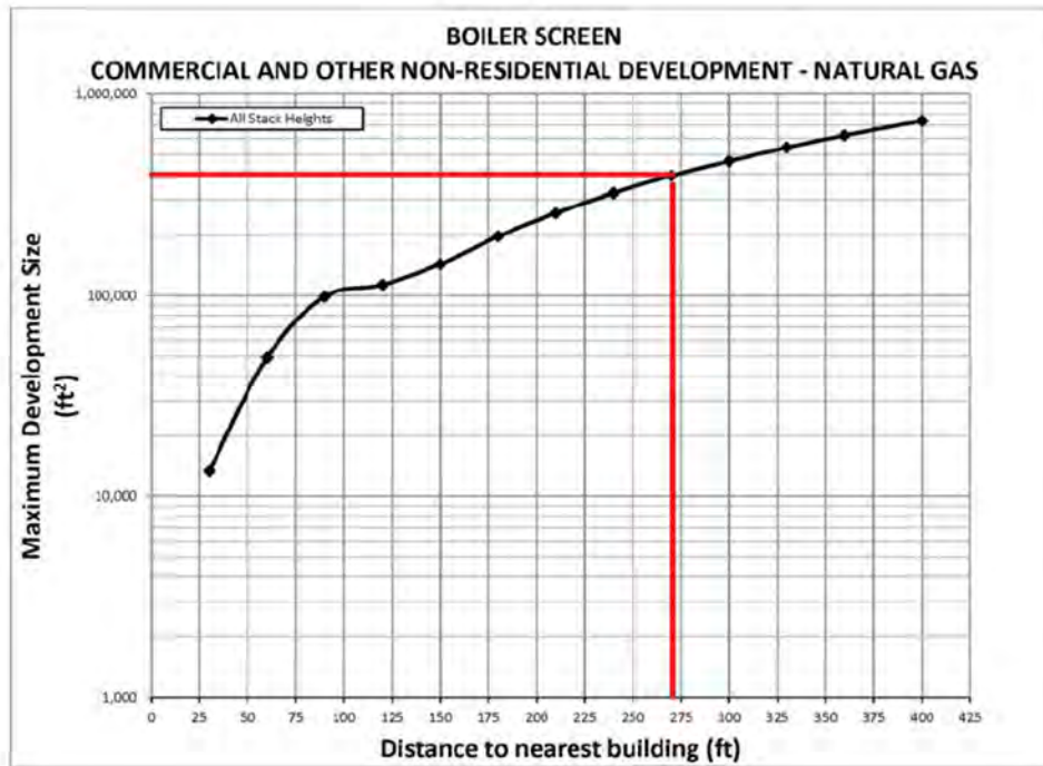
Figure 14-1 CEQR Boiler Screen Nomograph
